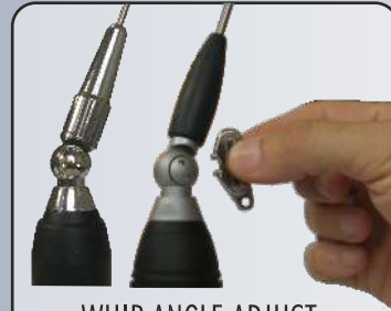
WHIP ANGLE ADJUST WITH SPECIAL KEY
