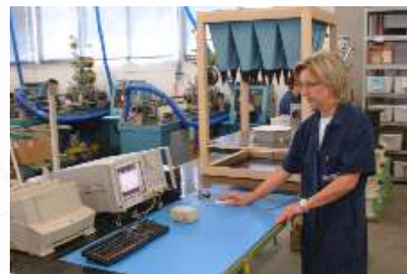
Final test with network analyzer
