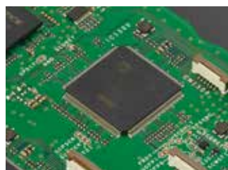
For band scope ADSP-21363 clock @332MHz
