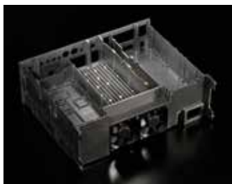
The position of the heatsink in the center of the rear panel
